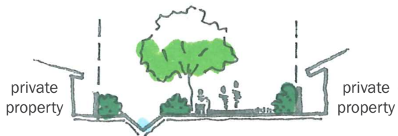
screen concrete shared screen path culvert planting
